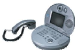
Aethra Theseus™ is a compactly designed videophone that offers ISDN 64K and IP-based video conferencing over BGAN. Theseus has been tested successfully over BGAN streaming IP as well as BGAN ISDN, and fully conforms to the H.320, H.323 and H.263 international standards (with transmission rates up to 384kbps over IP).
