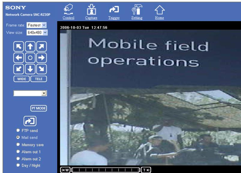
You can select the Frame rate where FPS indicates "the no of frames transmitted per second", and change the view size of the image.
