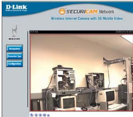
Using the **Connection Type** option, you can select whether to get an audio plus video feed, or one feed only. In addition, you can select the transport protocol. Inmarsat recommends that you use UDP for Streaming IP data connections, and TCP for Standard IP data connections.
