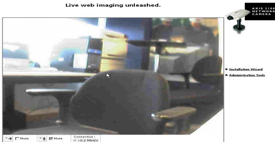
The main page contains the Installation Wizard and Administration Tools. The Installation wizard enables you to create the users and define their passwords to prevent any unauthorized use. The AXIS 2100 supports multilevel password protection, where access is strictly restricted to defined users only.
